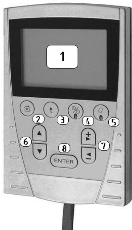
Fig.no.1 Service elements of HMI unit for Saphir regulator control
